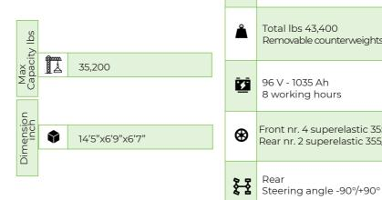
Front-wheels drive. 2 electric motors AC 10 kW 96V Insulation class H Total lbs 43,400
